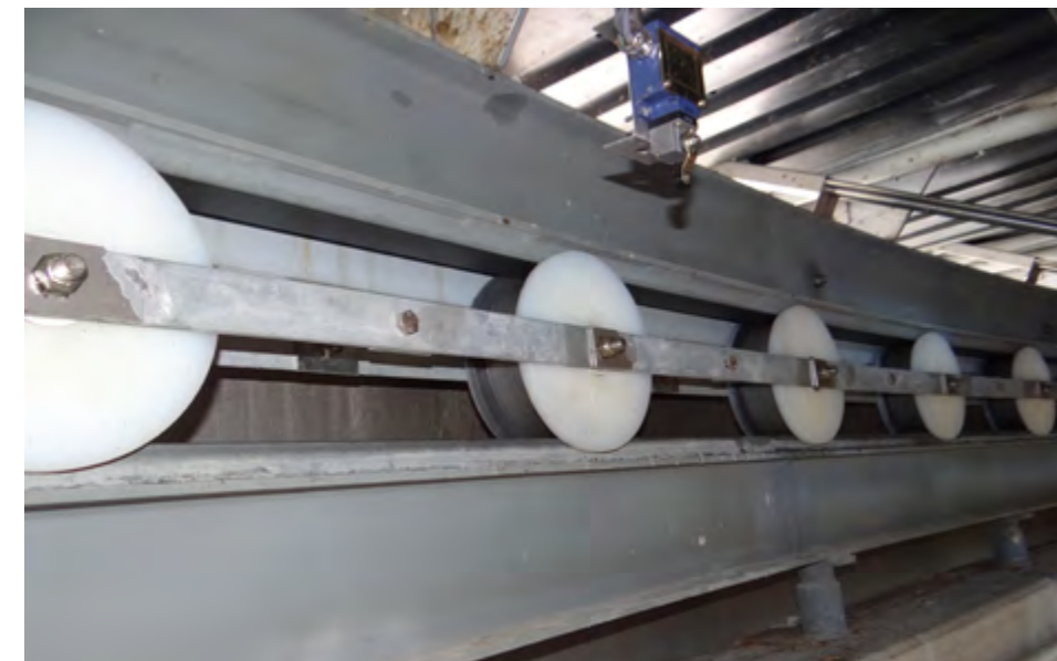
Self-tracking patented nylon multiroller system
