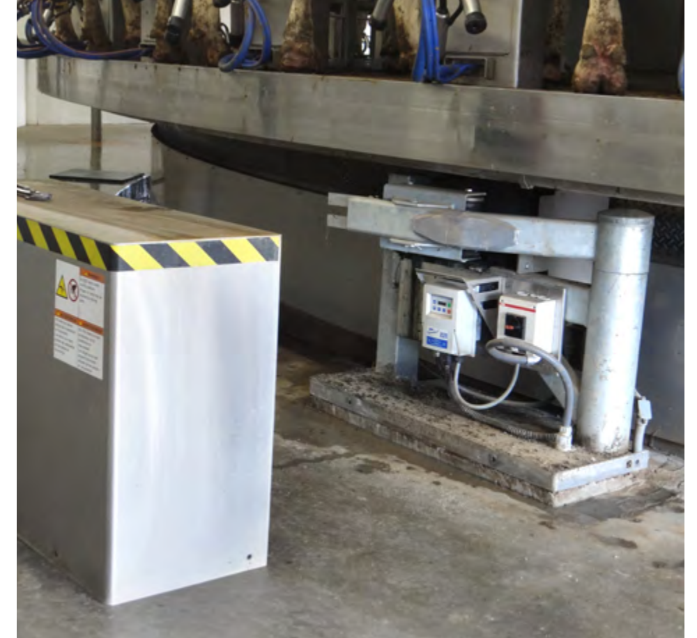
Drive unit – easy to service and installed in redundancy for back-up protection.
